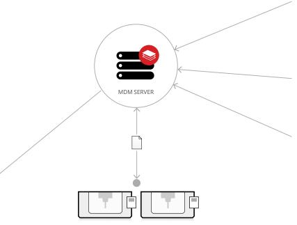
TRANSFER FILES TO/FROM MACHINES OR REMOTE REQUEST DIRECTLY FROM THE CONTROL
